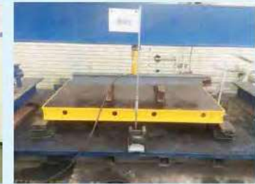
Panel Loading Capacity Test
