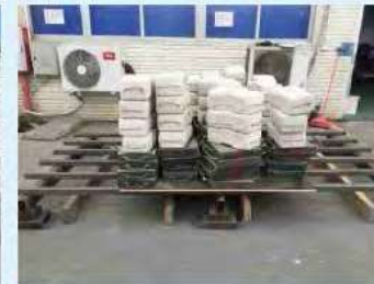
Loading Capacity Test
